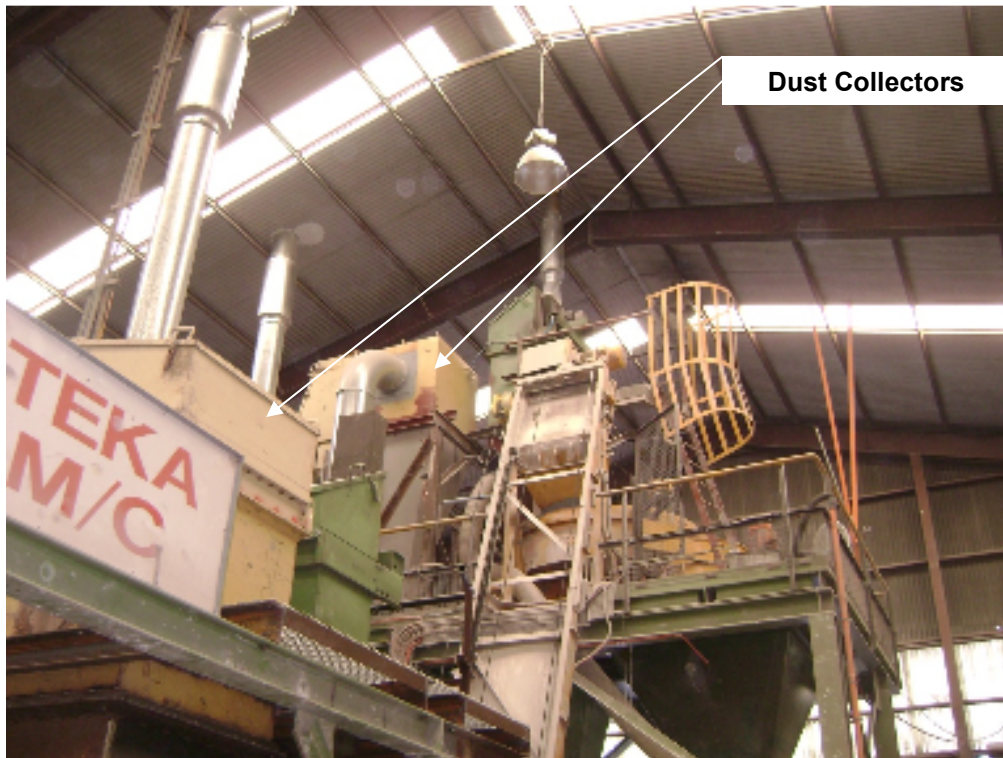
- Diagram 7 - Vesuvius Bulli Refractory Plant – TEKA Machine Typical Arrangement for Dust Collectors at back end of Plant Process
