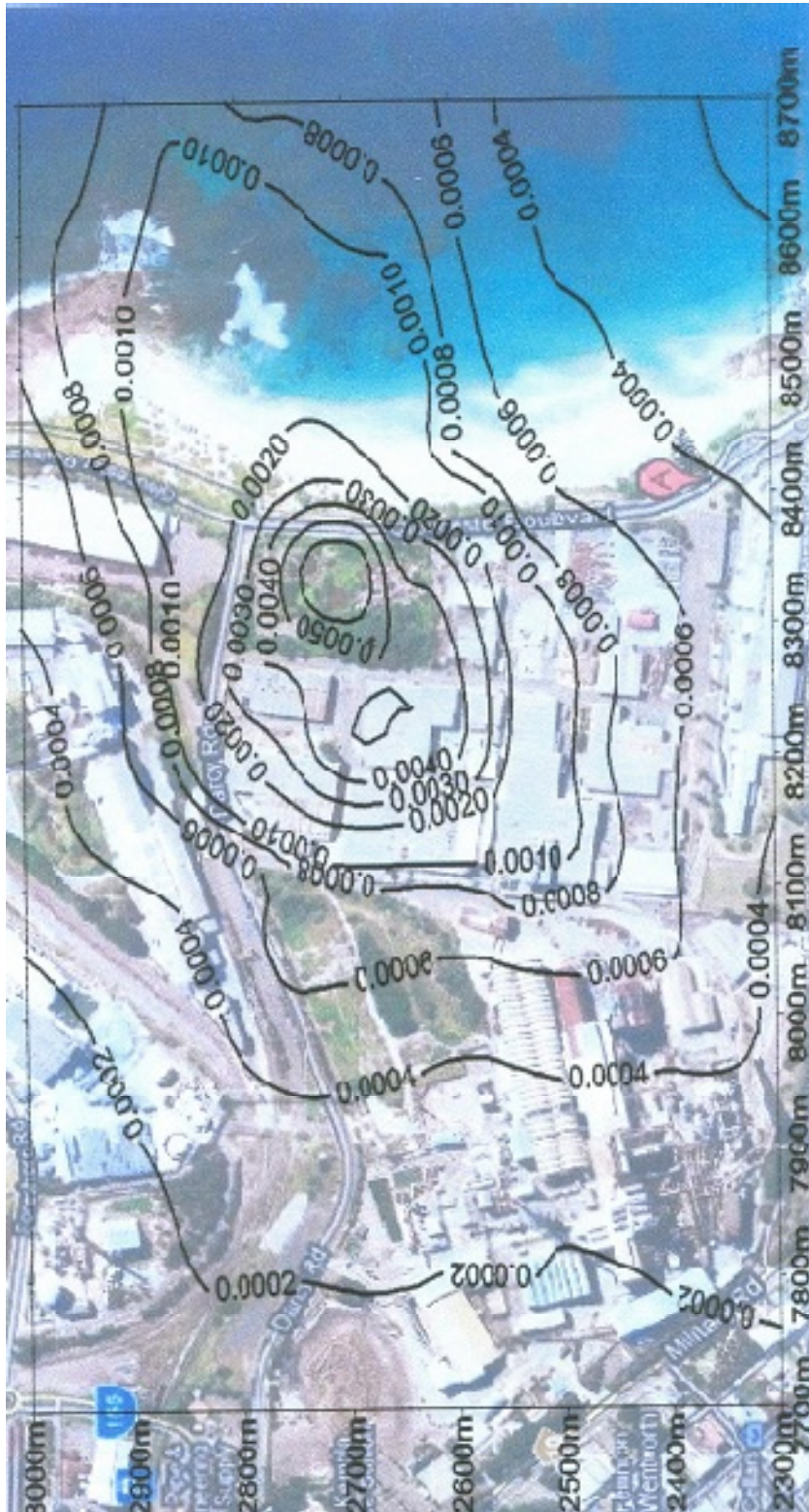
Diagram 6 Predicted Dispersion of Phenol from Plant (Concentrations in micrograms/m 3 – 99.5% average)
